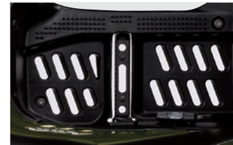
Full floorboards with drain holes
